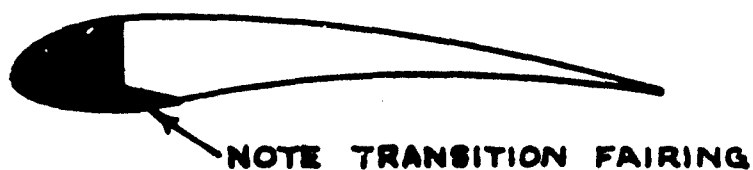
NON-DROOPED SPAR PROFILE (LOADED)
