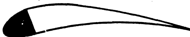
DROOPED SPAR PROFILE (LOADED)
