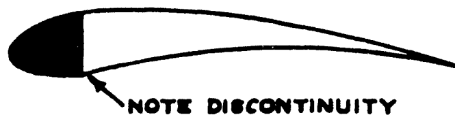
NON-DROOPED SPAR PROFILE (LOADED)
