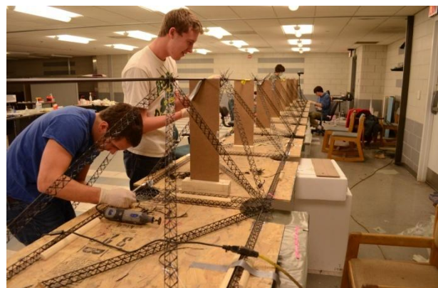
Figure 31: Assembly jig for one airframe truss arm.
