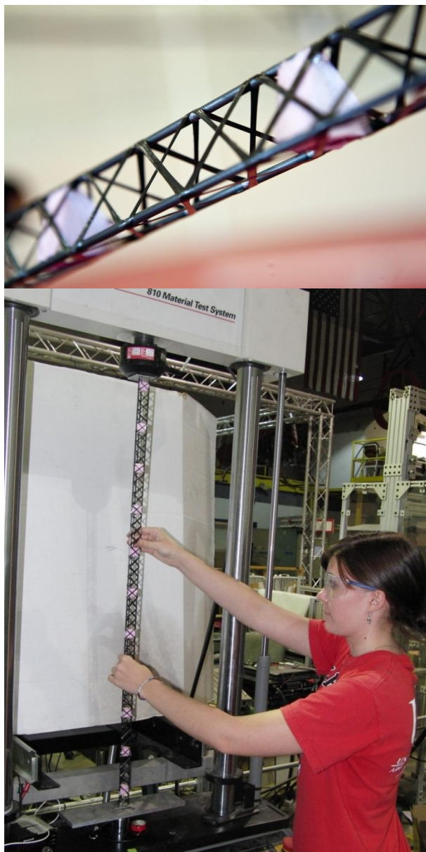
Figure 20: Detail of micro-truss structure (top) and micro-truss under compression testing (bottom).
