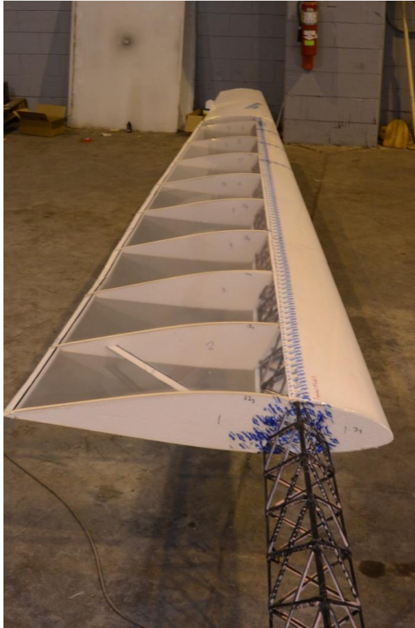
Figure 38: Gamera II blade with full-chord foam shell at the tip.
