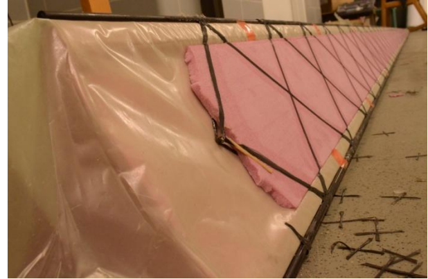
Figure 33: Gamera II spar with foam plates after filament-winding, vacuum bagging, and room-temperature curing process.
