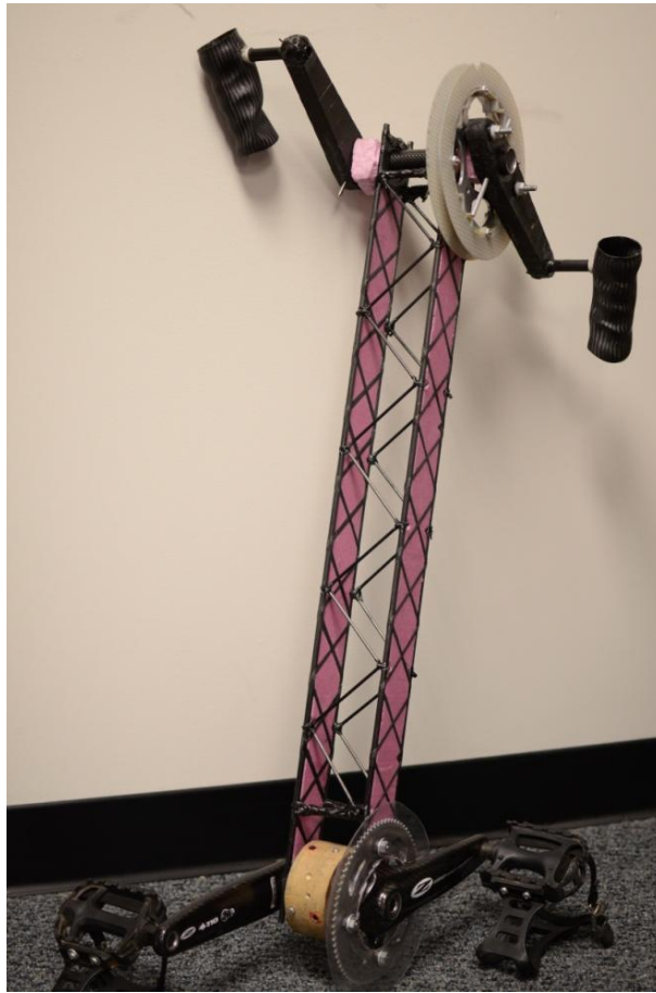
Figure 29: Box-truss cockpit core concept with hand and foot cranks mounted.
