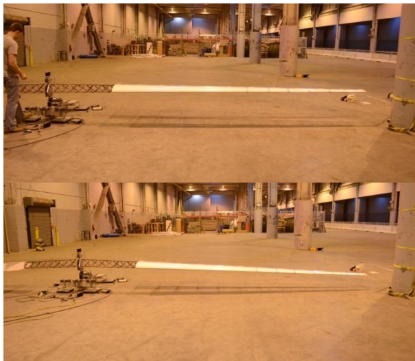
Figure 39: Testing the effect of negative pre-cone (top: baseline, bottom: -3^\circ ) on hover performance.
